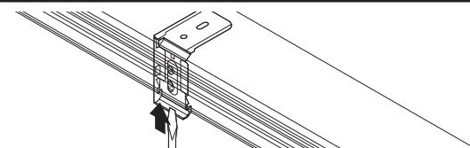
Center stack. Apply pressure to bottom of bracket with screwdriver.
