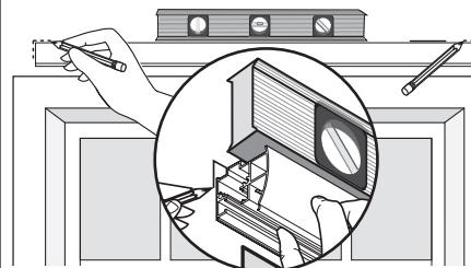
Align top of headrail to marks made. Center over window/door. Mark corners. Measure in 3" from each end and mark bracket locations. Space additional brackets evenly if required. See bracket usage chart in step 1.
