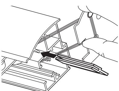
Slide the proper number of **CORD RETAINERS** onto the first tab behind the front of the headrail. Space evenly down the length of the headrail. See table below for the proper number to install.
