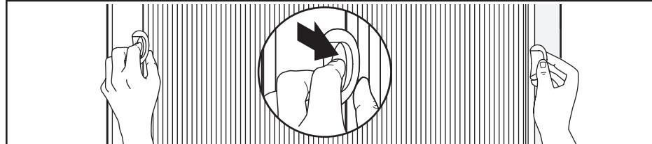
Press release buttons on handles to operate shade or equalize cord tension.
