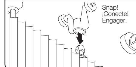
Shade may be shipped with wheels detached from the fabric. Snap together as shown.
