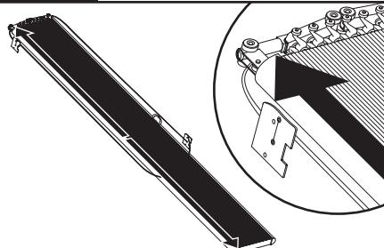
Remove plastic wrap and measure the length of the side rails. Record this dimension.
