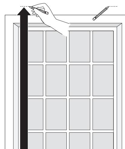
If using projection brackets measure up from the floor the dimension from step 2 and add 2-1/4". For direct wall mount, without projection brackets, measure up from the floor the dimension from step 2 and add 2". This will provide approximately 1/4" clearance under the shade. If additional clearance is required add it to the dimension calculated above.
