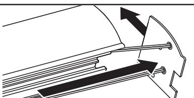
Ensure cords are not twisted. Thread cords along headrail grooves.
