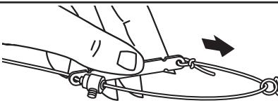
Make sure the tension plate is slid down against the locking collar.
