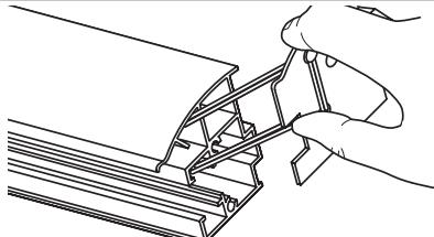
Hold right end plate slightly above position on end of headrail. Cords will be under tension.
