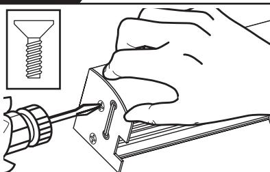
Keep shade assembly to far left ensuring cords are not caught between screws and plate. Secure left end plate with two screws.
