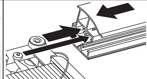
Lay headrail and shade assembly on a clean flat surface, front face up. **Carefully free cords from packaging; untangle if necessary**, and place on top of fabric. Press release buttons on handles and open shade to approximately 14". Starting with the **LEFT** end of the headrail, slide the headrail onto the shade assembly.
