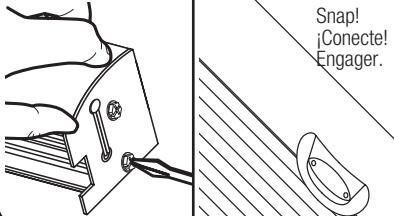
Secure right end plate with two screws. Clip plastic end caps over both end plates.
