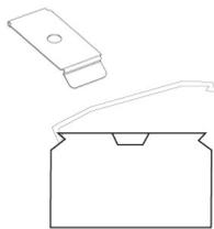
Use mounting clips to secure headrail on ceiling or inside mounts. The center of the mounting clips align with the center of the louver carrier stem. Position the screws a minimum of 2 1/4" in front of the window frame or any projection.
