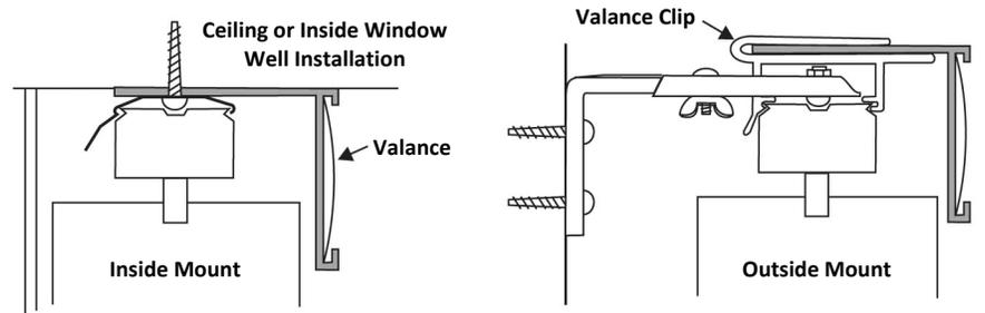
For Outside Mount Installations, use the following # of Valance Clips based on the Blind Width:
