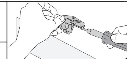
**\*Note:** For blinds under 13-7/8" wide, or all same side control blinds, brackets must be positioned directly over the blind internal tilting components
