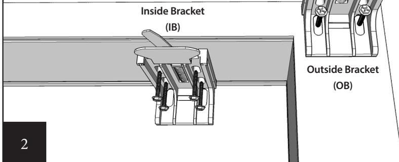
**2****Installing the Shade into the brackets**
