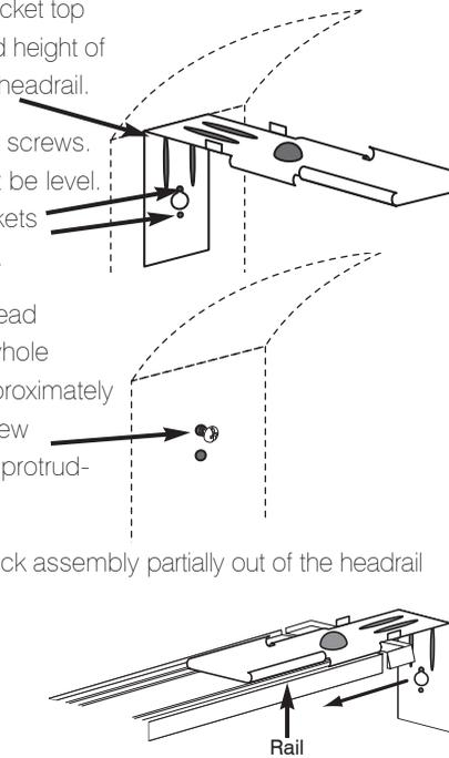
6. Hook one bracket onto the screw in the window frame, using the keyhole slot. Bring the other end bracket over the screw at the other side of the frame. Slide down, flexing bracket inward until the screw engages in the keyhole slot.
