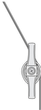
Mount the cord cleat at a safe height, taking into account furniture or other objects upon which a child may climb. Then, after each use of the shade, simply wrap the excess cord around the cleat. It's fast, easy and safe.
