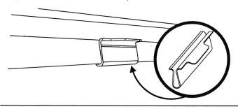
Attach the handle to the bottom of the shade as illustrated. The handle is designed to minimize contact with the shade fabric. Always raise and lower the shade slowly to assure that the fabric gathers neatly.
