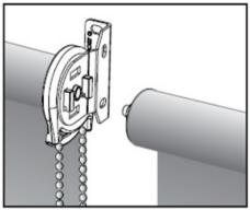
Note: If sharing a bracket between two shades, bracket can only be shared by a clutch and a pin end, not a clutch-to-clutch or pin end to pin end.
