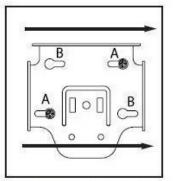
Slip the mounting bracket over the two screws and slide the bracket sideways until the screws heads capture the bracket.
